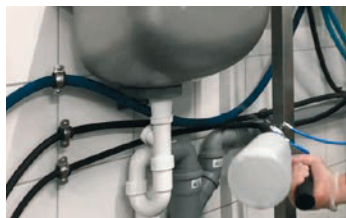
Partial cleaning: Also used as a handheld device, contaminated surfaces can be easily reached with the cold mist.
